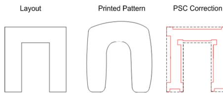
Figure 15. Layout, Printed Pattern and PSC Correction for U-shaped structure
