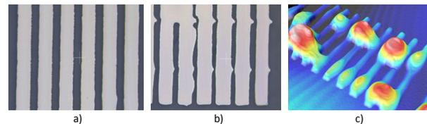
Figure 12. a) Correct spacing, b) Printer misalignment, c) Electrical shorts
